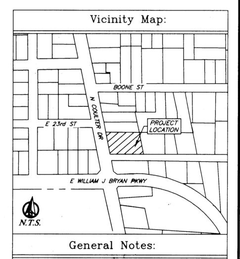
Coordinates and Bearing System shown hereon are NAD83 (Texas State Plane Central Zone grid North) based on the published coordinates of the city of Bryan Control monument GPS-33 (N:10230645.06; E:3550917.70) and as established from gps observation.
